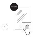
Use the CC-240 sandpaper to sand the surface of your cabinet. Sand the top surface until there is visible sand marks in the surface. Please pay attention to sanding the corners.
